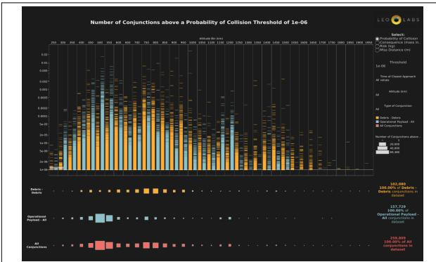
Fig. 1. The nearly 260,000 conjunctions captured by LeoLabs in the first half of 2022 (i.e., as of 30 June 2022) highlight the growing STM areas of interest between 500 to 600 km and lingering SDM concerns in spots from 700 to 850 km. Secondary peaks for STM and SDM are at ~1,200 km and ~1,400 km, respectively.
