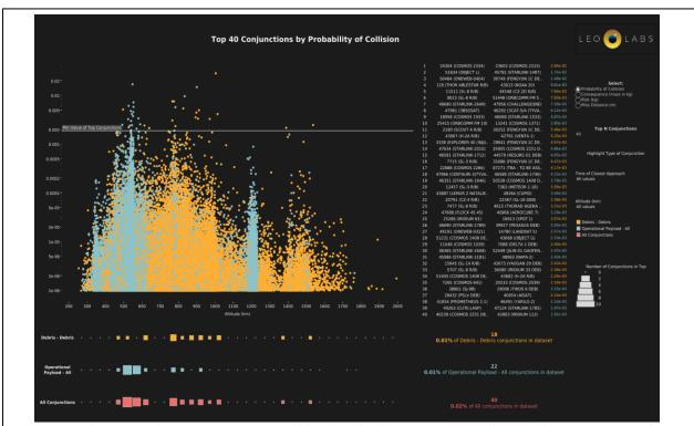
Fig. 2. The PC for the top 40 events plotted by altitude shows an apparent balance between SDM and STM events (i.e., roughly equal numbers of events out of the top 40 highest PC conjunctions).
